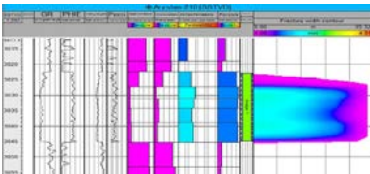
Figure 5. Fracture created during Calibration test, built on calibrated reservoir, before main job
